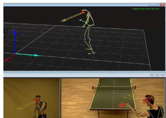
Collect and visualize eye tracker data in QTM. The data is visualized as a gaze vector with a maneuverable vector trace
