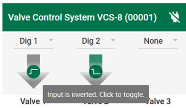
Assign valves to digital input ports via the drop down menus. Each valve can be assigned to any of the 16 Digital In bits (D-Sub25) or the Trig/Sync input (BNC). Digital inputs can be used "as is" or "inverted". If a digital input has been assigned to a valve, the valve will directly reflect the logical states on the digital port:
