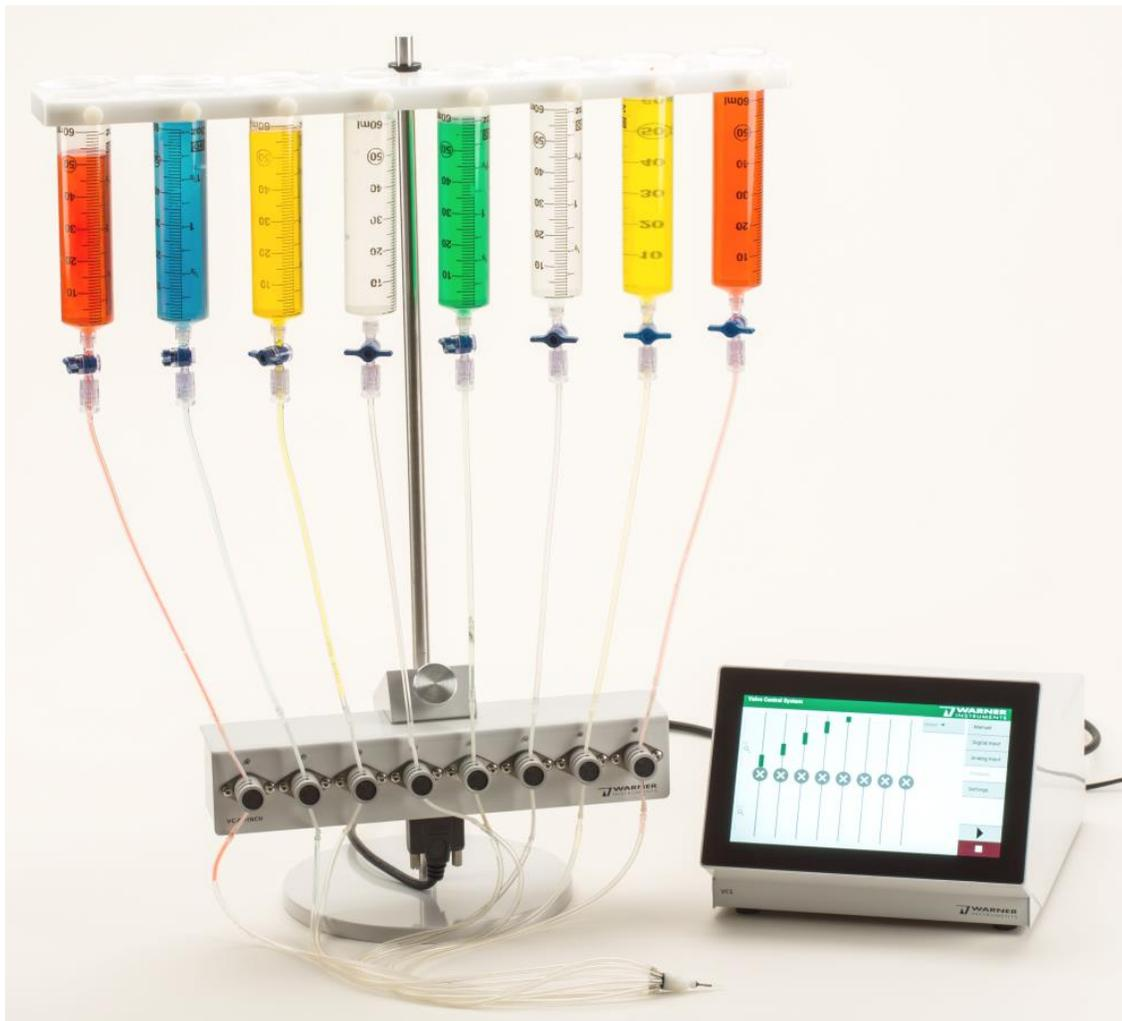
The Valve Control System (VCS) is a multivalve perfusion system designed to automate and control the delivery of solutions to imaging and recording chambers. Its flexible design also allows the VCS to be used in many diverse applications. Warner Valve Control Systems are configured to control six or eight Pinch or PTFE valves.
