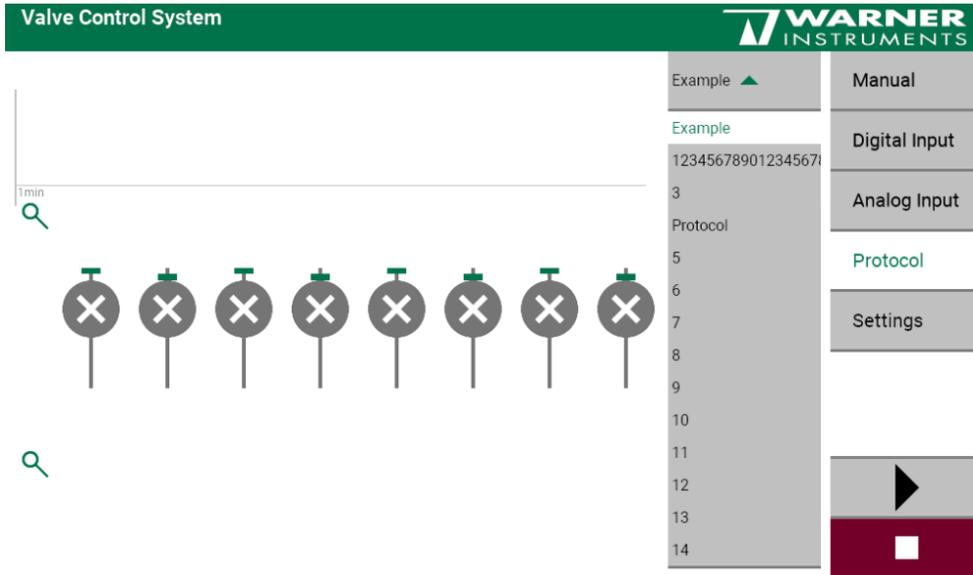
Select the desired protocol from the drop down menu. The protocol should be downloaded onto the control unit, if it should be processed without computer connection.
