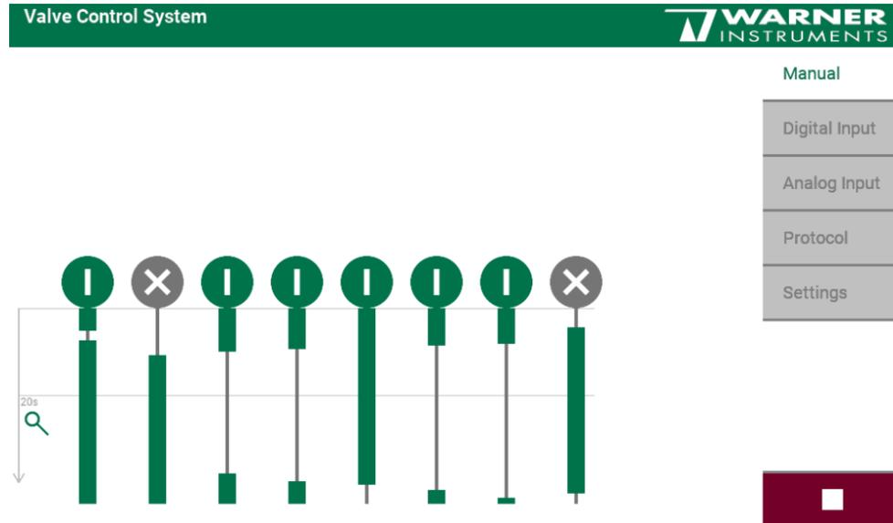
Each valve can be controlled individually by clicking on its circular icon or start and stop or all valves can be started and stopped together via "Start" button. Use the "Stop / Emergency" button to immediately close all valves, if needed. Green circles with a vertical line indicate an open valve, gray circles with an "X" indicate closed valves.
