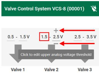
In order to open a valve continuously, set the lower analog input threshold to a value higher than the upper analog input threshold.
