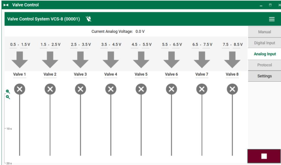
Connect the analog input port on the back side of the device. Define the voltage range in which the respective valve should be open. Change the default voltage threshold ranges of the valves by using the "Plus" or "Minus" icon or by overwriting the numbers.
