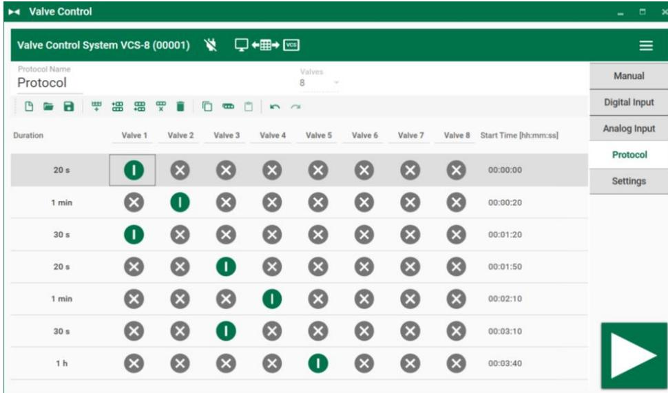
For example, a simple protocol might consist of first opening both valves 1 and 3 for 10 seconds, then closing valves 1 and 3 and opening valves 2 and 4 for an additional 30 seconds.
