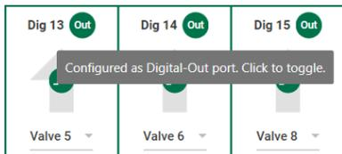
The purpose of a digital in port is to receive a control signal in "Digital Input Mode" and is used to control one or more valves by opening and closing while synchronizing them to state changes in the control signal. See the section "Digital Input Mode" for more details. If a digital out port is assigned to a valve, then the port's state reflects the state of the valve. It is possible to configure if the valve's state should be presented "as is" on the digital out port or as "inverted":
