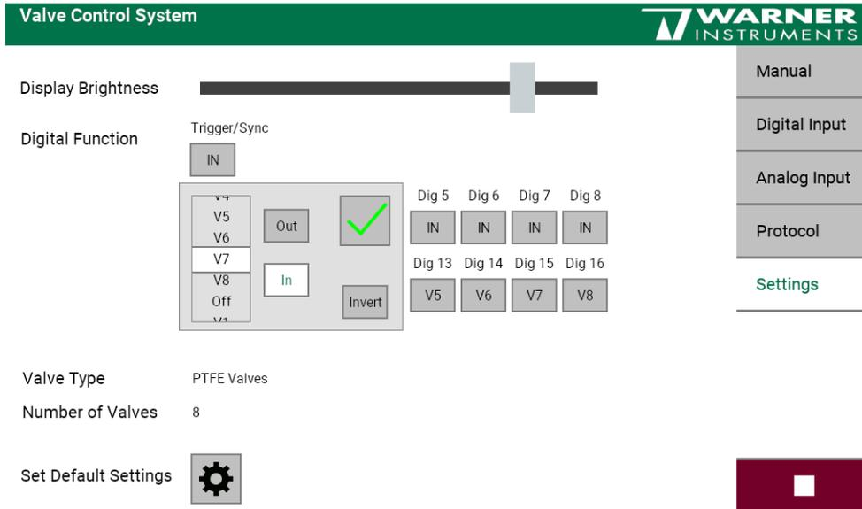
The "Settings" menu on the touch screen has two additional functions in relation to the software "Settings": Adapt the "Display Brightness" with the ruler above and "Set Default Settings" with the button below. In addition the "Valve Type" and the "Number of Valves" is displayed.
