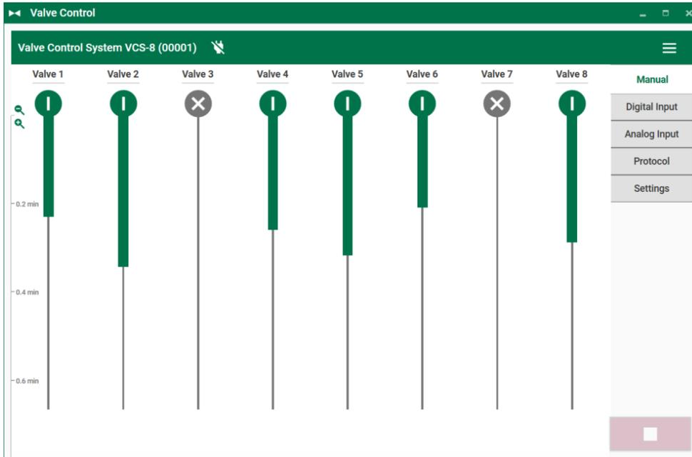
Valve states can be toggled between open and closed by either clicking the valve symbol or with the keyboard shortcut "Ctrl + the valve index". For example, pressing **Ctrl + 3** will toggle the state of valve 3. Open valves are indicated in green, closed valves are gray.
