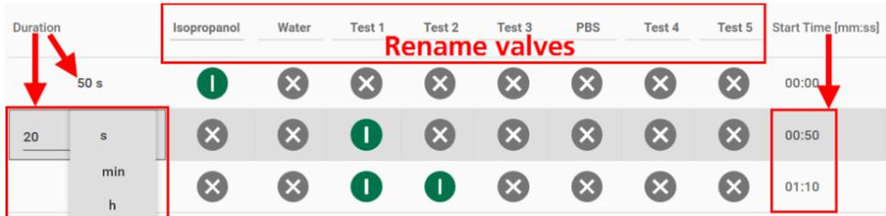
Click the valve header with the right mouse to cut this name of the valve, to copy and to paste it into another column.
