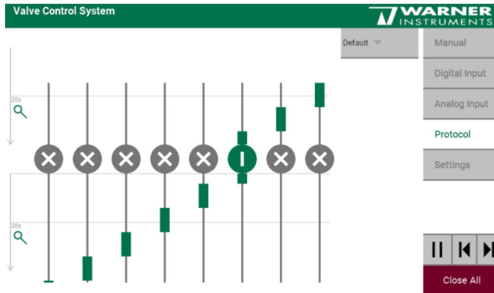
Start a protocol with the "Start" button. The "Start" button is replaced by the "Stop / Emergency" button in red and the "Pause" and "Skip to Next Step" and "Skip to Previous Step" buttons in green. So it is possible to jump from one step to the next or back to the step before or to pause the protocol.
