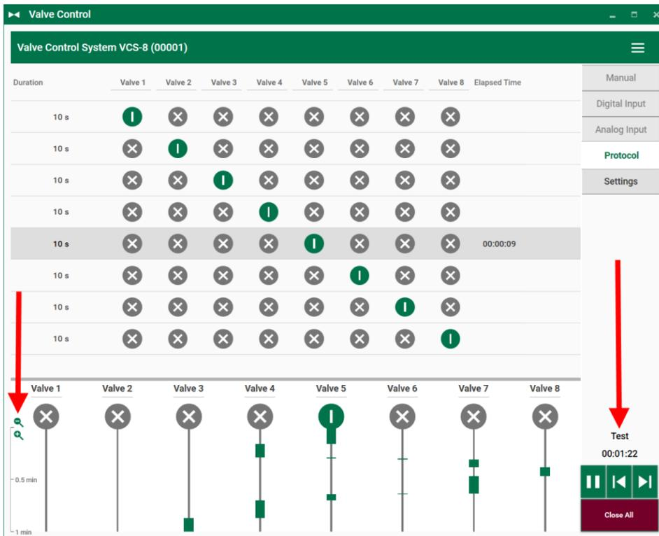
Select a protocol and start it with the "Start" button. The "Start" button is replaced by the "Stop" button in red.
