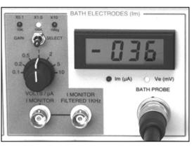
When in clamp mode (<u>CLAMP</u> MODE SELECTOR switch set to *slow* or *fast*), the CURRENT METER displays the current ( $I_m$ ) sensed by the bath electrode. A lit LED indicates current readings in  $\mu A$ .
