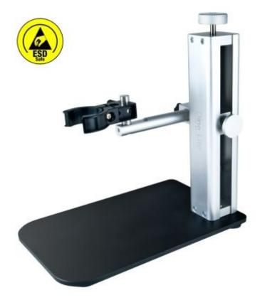
The Dino-Lite RK-10A is a sturdy and stable high-end stand solution that can be used with all the professional Dino-Lite models. It is constructed of resilient stainless steel and lightweight aluminum and offers a very precise fine-focus adjustment as well as a quick release function.
