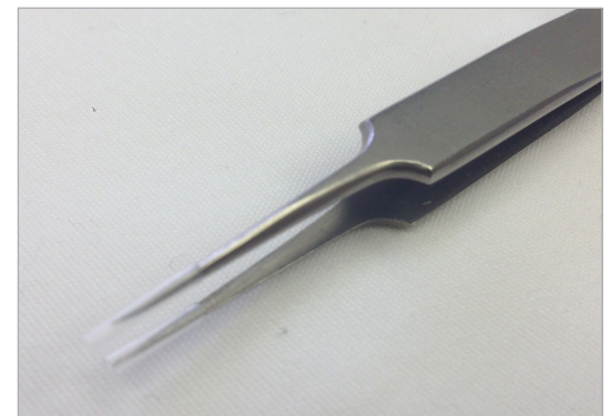
Place polyethylene tubing over the forceps' tips to protect the Catheter body from damage.
