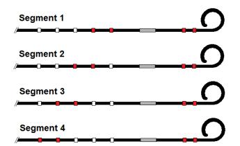
Four selectable segment lengths (active rings in red). Segment 1 is the shortest (for smaller hearts) while segment 4 is the longest (for larger hearts). The distal electrode pair (1 & 2) remain the same for all segments.
