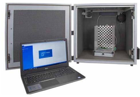
ANY-maze controls the shocker, the sound generator and the light (I.R. and visible), and automatically detects the animal freezing, reporting information such as: total freezing time, number and duration of freezing episodes, latency times between stimuli and freezing events.
