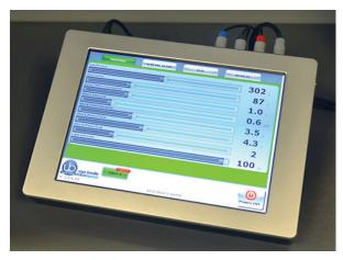
The Unit, incorporating a 12" touch-screen, manages the Passive Avoidance Test via the **40550-010** Software. Up to 4 cages can be connected to the same Controller. If more than one cage is connected, an expansion box **40500-005** is required for each additional cage.
