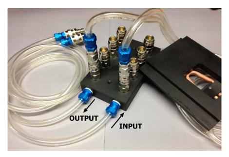
After connecting the tube to the mechanical stimulator, fix them into the brackets provided, as shown on the picture on the right.
