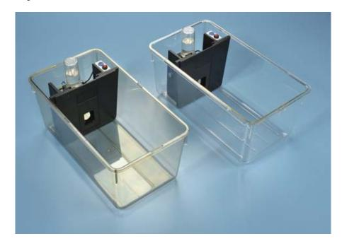
The **thermal stimulator** relies on a copper tubing loop and a circulating water bath, whose temperature can be adjusted from ambient to 70°C, to reach hot nociceptive threshold.
