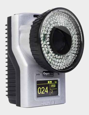
Oqus Video (also known as Oqus 210c) is a synchronised and dedicated video camera that can be calibrated together with an Oqus motion capture system, providing a video image that is fully synchronised with the mocap system.
