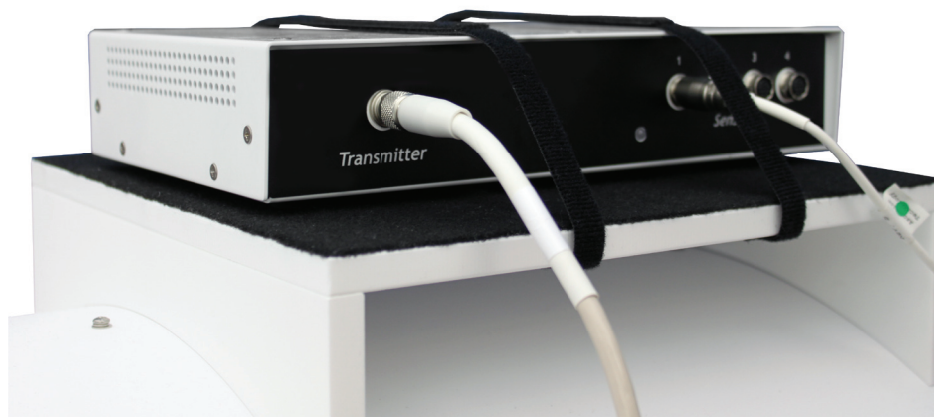
Figure 3 Completed Installation — shelf mounted with MoTrak
