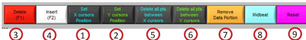
**Set X Cursor Position (1):** The Set X Cursor Position brings up a window through which the user can set the high and low position of the X cursors by changing their numerical value. The Cursor Pos X Low and Cursor Pos X High show these settings.
