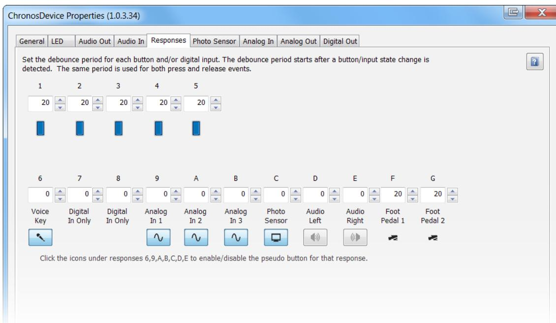
Note that in the second row of responses, the digital inputs 7 and 8 do not have an icon beneath them. This indicates that they are not mapped to system-defined pseudo button response. However, if the I/O Expander were used to collect a digital input on the pins that correspond to responses 7 or 8, then E-Prime would register that input as a 7 or 8, respectively.
