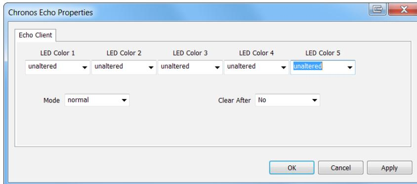
The Chronos Echo Properties dialog provides access to each individual LED. The default value is “unaltered”, which indicates that the LED’s color setting will not be altered in response to a button press or release. To change the color of an LED when its corresponding button is pressed and/or released, select a color from the dropdown list for the LED of interest. The color to be echoed can also be set from an attribute reference.
