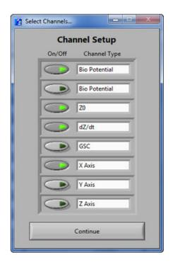
From this screen the user can specify which channels will be used for acquisition. Up to four channels can be selected simultaneously. If any more than 4 channels are selected, a warning will appear and the most recently selected channel will be automatically deselected. When all desired channels have been enabled, press **Continue** to return to the Network Device Detection screen.
