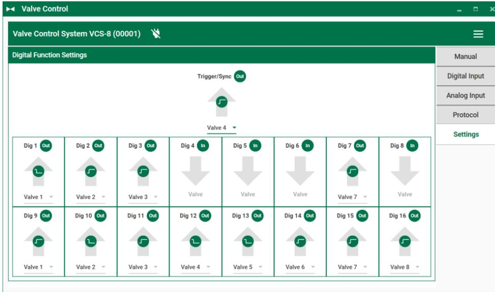
You configure the digital ports via the "Settings" menu. Two digital connectors are available on the rear panel of the control unit: "Trigger/Sync" and "Digital In".
