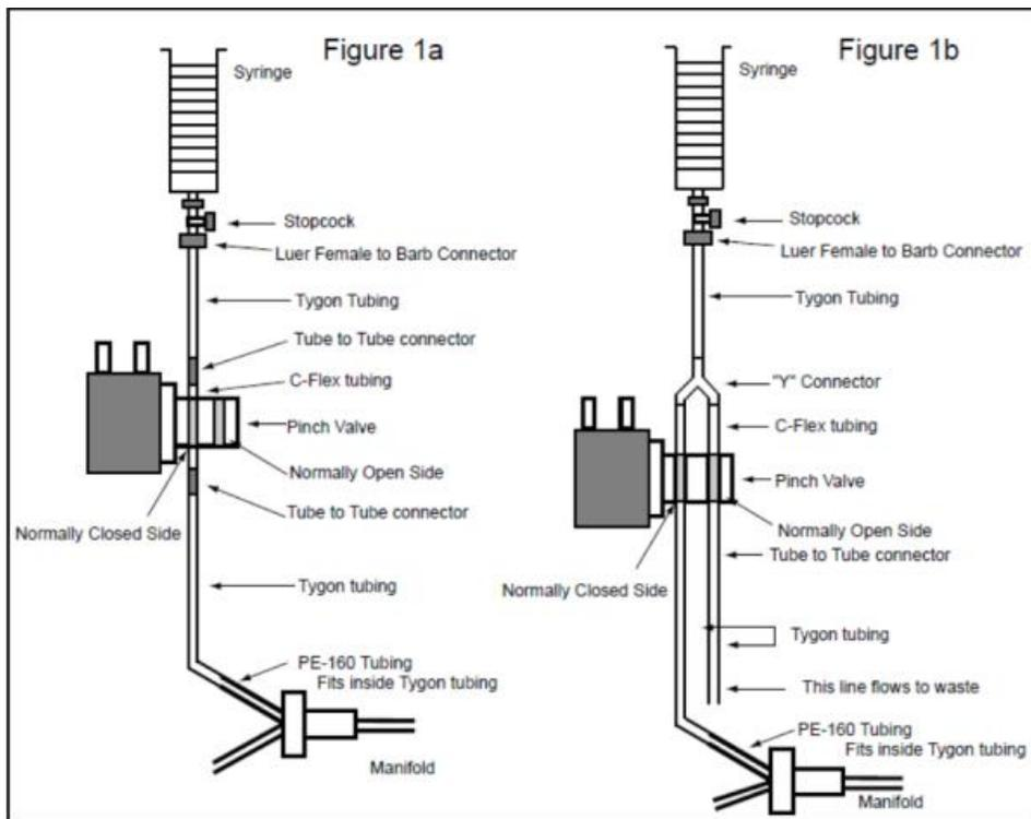
Note: Minimizing the length of C-Flex® or silicone tubing used will reduce the gas permeability of the system.
