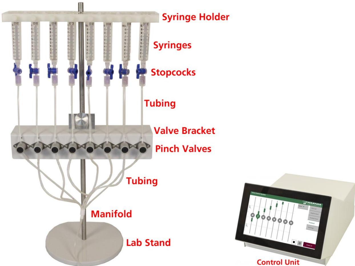
The complete VCS Pinch Valve System includes a control unit, a lab stand, a valve bracket with valves and connecting cable, C-Flex®, Tygon, and PE tubing, an MP Series manifold, six or eight 60 cc syringes, a syringe holder, and an assortment of tubing connectors.
