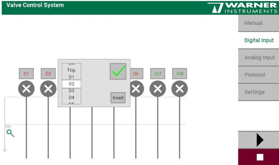
Connect the digital input port on the back side of the device. Assign valves to digital input ports via the drop down menus and determine if the digital input should be used "as is" or "inverted". Inverted valves are indicated in green letters above the valve icon. If a digital input has been assigned to a valve, the valve will directly reflect the logical states on the digital port:
