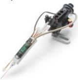
Easy luer-lock connections and manipulator mounting. Thermodynamic design maintains temperature with 5 ml/minute flow from both tips without any metal tubing.
